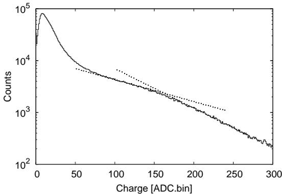
Figure 1: Charge histogram for one minute of data of a  $4\text{ m}^2$  detector at Sierra Negra. While there is no characteristic muon peak at this altitude, a change in the slope can be determined and used for calibration. The intersection of the two fitted dotted lines is used to determine a calibration reference point.
